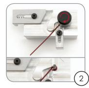
Place the large peg in place, and then rotate it clockwise to form a loop. To add a bead, eliminate this step.
