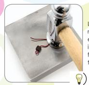
Lightly hammering the rounded part of the earring hook will make it stronger, and keep it from straightening with the weight of the beads.
