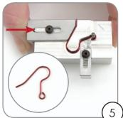
Push the large piston to guide the wire to obtain the hook shape. The small piston can be used to hold the wire in its place. Cut any excess wire, if necessary. To make your hooks more comfortable to wear, use the wire rounder to round off the sharp tip of the wire.
