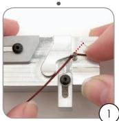
Cut a 5 cm. length of wire. Place one end in line with the line indicated on the Fishhook maker. Using your index finger, curve the wire slightly towards you.
